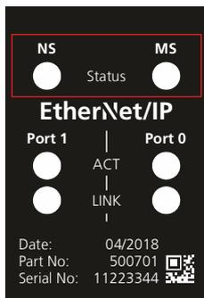
Figure 10: EtherNet/IP™ status LED's
