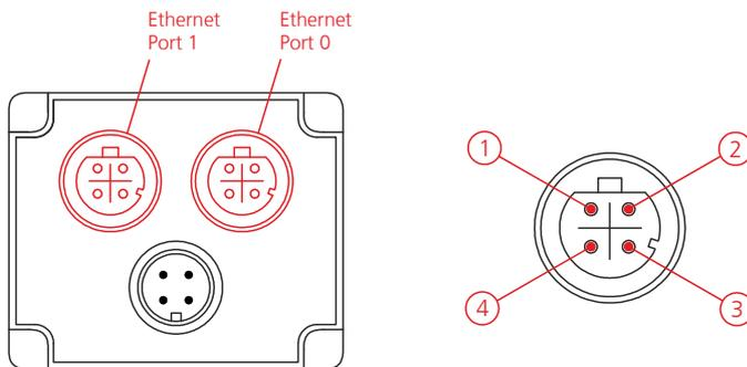
Figure 4: Connection diagram of the Ethernet port 0 & 1
